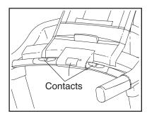
To measure your heart rate, stand on the foot rails and hold the metal contacts on the handrail for approximately ten seconds—avoid moving your hands. When your pulse is detected, several dashes will appear in the display and then your heart rate will be shown. For the most accurate heart rate reading, continue to hold the contacts for about 15 seconds.
